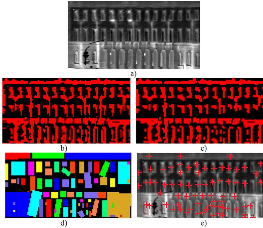
Fig .4 Region detection: a) input b) extraction of candidates for windows from IR texture using local dynamic threshold; c) separation of the regions and removing false detections using morphological operations; d) rectangular bounding boxes for the extracted regions; e) gravity centers
